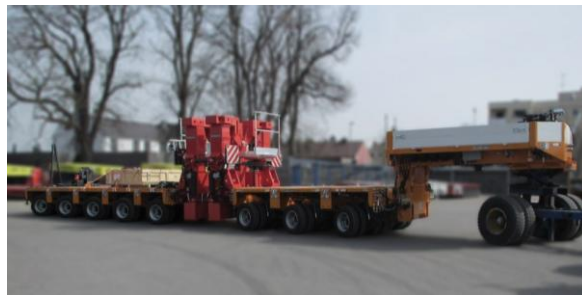
Tower Adapter / Currently located in Africa – 30 tons per axle
