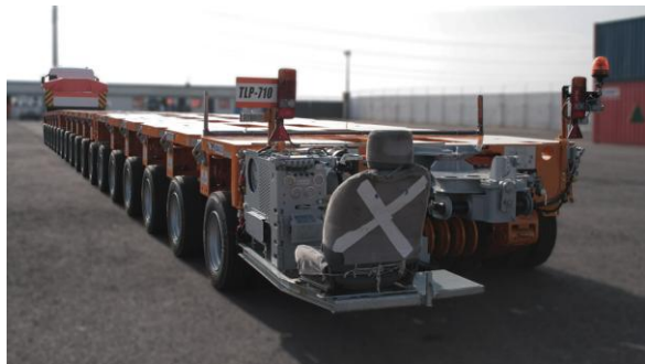
Modular trailers set up as per project requirements
