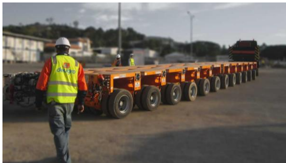
6 x 6 axles 30tons per axle
